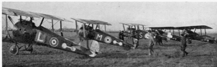
Not a railway advertisement, but Sopwith Camels lined up on an aerodrome in France. With the 300 h.p. Bentley rotary engine, the Camel was one of the best single-seater fighting machines in France in 1918.
